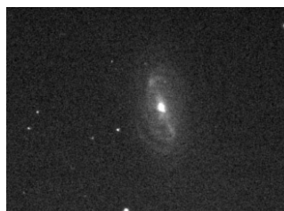
Field of View of TC-237 autoguiding through an 8" SCT at F/7. 30 second unguided image of the same area taken with the TC-237 tracking CCD demonstrates the benefit of having 2.7X the field of view: An increase in the number of potential guide stars. 328 x 247 pixels at 14.8 microns (binned 2x2).
